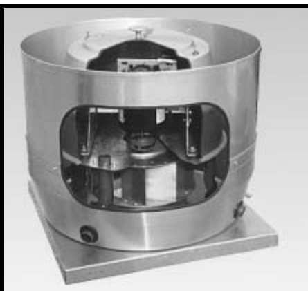
CUBA Belt C-Drive Upblast Centrifugal Exhaust PRV Sizes - 12 to 24 711 to 8850 CFM; Static Pressure to 2" AMCA Seal for Sound and Air UL705 or UL762 Listing Available
