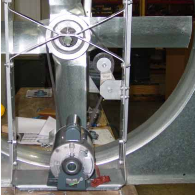
NEF36 with motor mounted at the bottom of the fan
