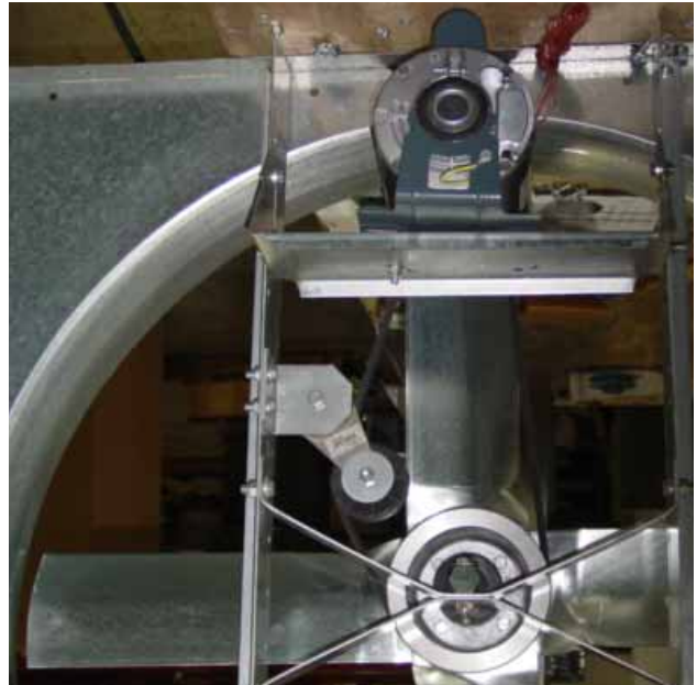
NEF36 with motor mounted at the top of the fan
