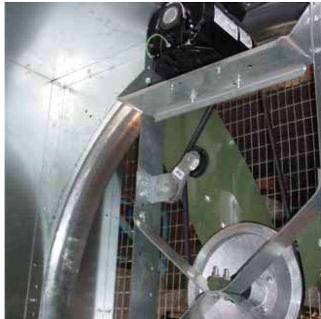
NEFB52 with motor mounted at the top of the fan
