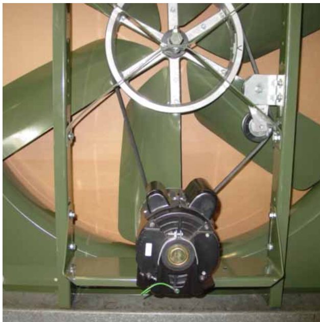
NBF42 with motor mounted at the bottom of the fan
