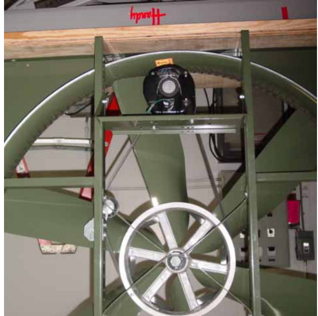
NBF54 with motor mounted at the top of the fan
