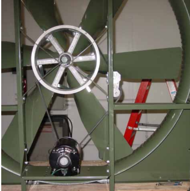
NBF54 with motor mounted at the bottom of the fan
