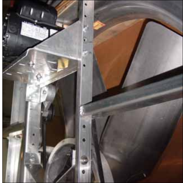
AL48 with motor mounted at the top of the fan
