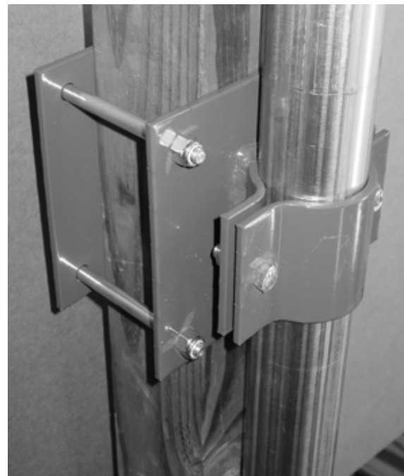
The pivot pipe is slipped through the wall pivot assemblies. Once in place, set the orientation of the fan and tighten all of the nylon insert nuts supplied to secure the unit.
