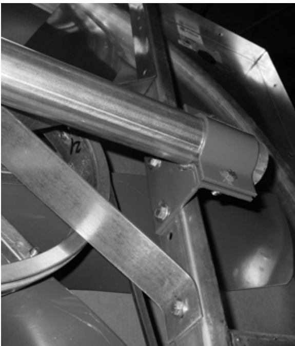
The pivot pipe is slipped through the two upright pivot assemblies. Do not tighten the hardware. Leave the hardware snug for now.
