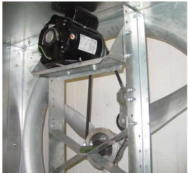
NBC36RM with motor mounted at the top of the fan
