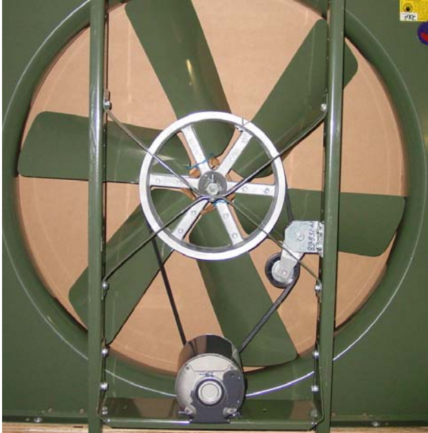
NBF36 with motor mounted at the bottom of the fan
