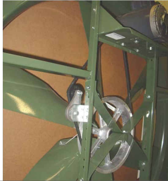
NBF54 with motor mounted at the top of the fan
