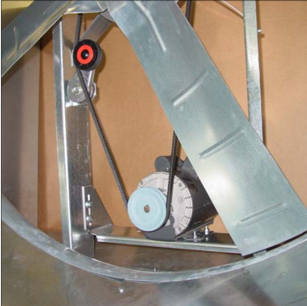
NEF54 with motor mounted at the bottom of the fan
