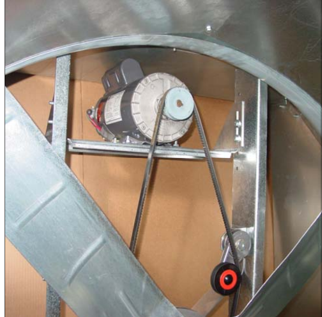
NEF54 with motor mounted at the top of the fan
