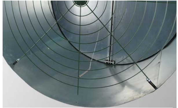
Figure 14 — Door Restraining Cable
